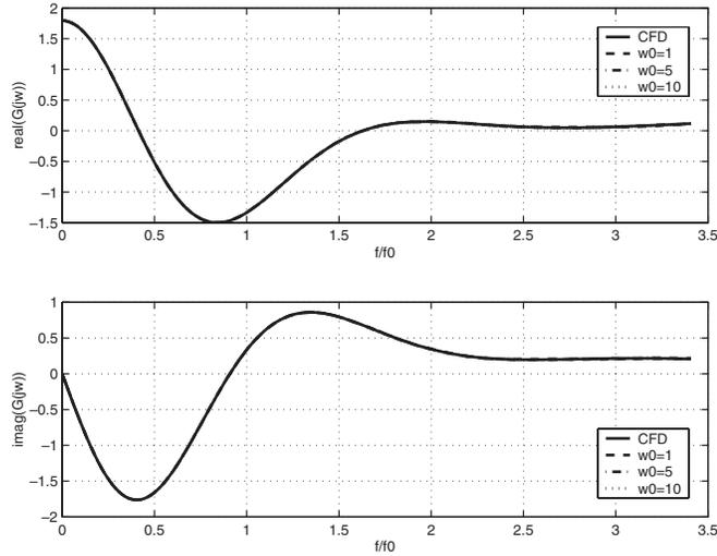
FIG. 4.6. Transfer function from bleed actuation to average throat Mach number for supersonic diffuser. Results from CFD model ( $n = 11,730$ ) are compared to reduced-order models derived using 200 Fourier coefficients with  $\omega_0 = 1, 5, 10$ .
