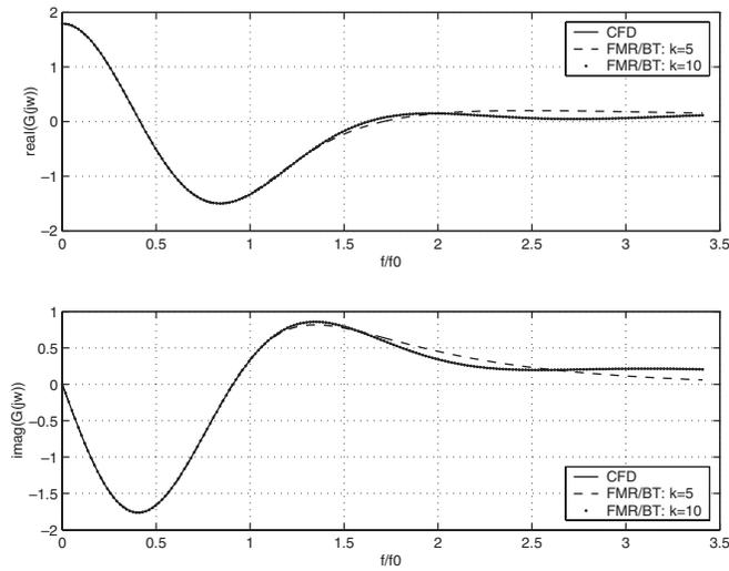
FIG. 4.9. Transfer function from bleed actuation to average throat Mach number for supersonic diffuser. Results from CFD model ( $n = 11,730$ ) are compared to reduced-order models with 5 and 10 states derived from the  $m = 200$  FMR model via balanced truncation.
