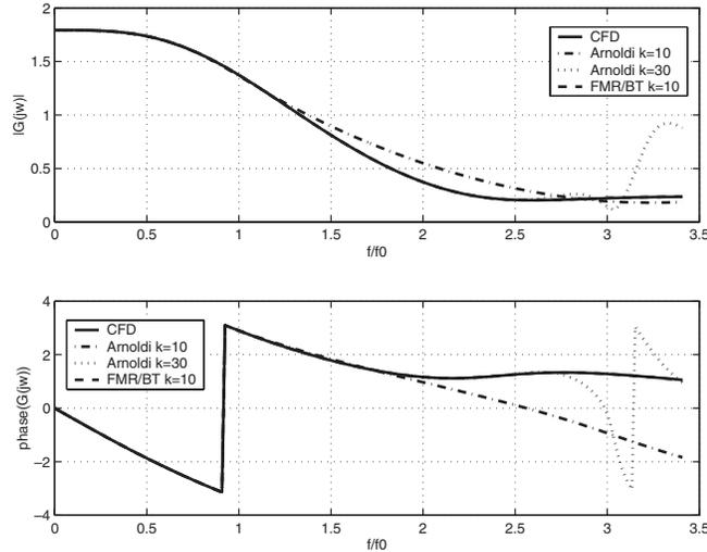
FIG. 4.10. Transfer function from bleed actuation to average throat Mach number for supersonic diffuser. Results from CFD model ( $n = 11,730$ ) are compared to an FMR/BT model with 10 states and Arnoldi models with 10 and 30 states.
