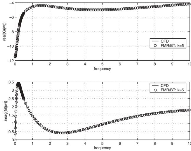
FIG. 4.3. Transfer function from plunging motion to lift force for subsonic airfoil. Results from CFD model ( $n = 13,928$ ) are compared to a fifth-order reduced-order model derived from the  $m = 200$ ,  $\omega_0 = 1$  FMR model via balanced truncation.
