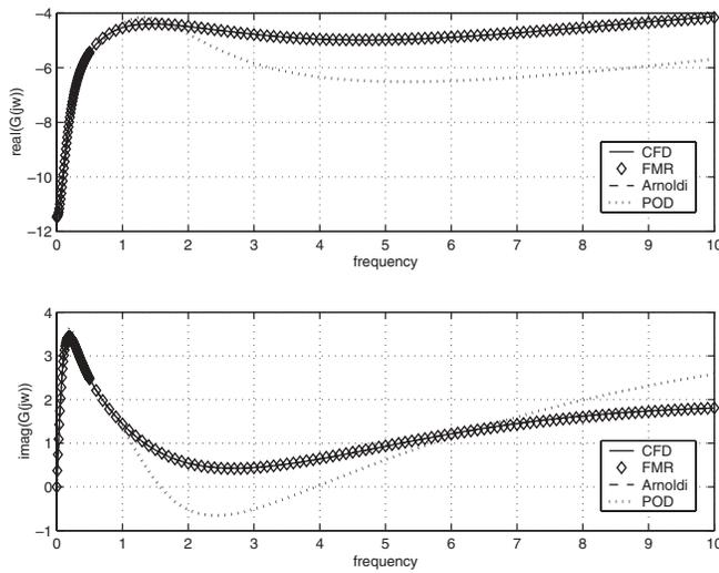
FIG. 4.4. Transfer function from plunging motion to lift force for subsonic airfoil. Results from CFD model ( $n = 13,928$ ) are compared to fifth-order reduced-order models derived using FMR, Arnoldi and POD. Both the Arnoldi and FMR models have been created using balanced truncation from an  $m = 200$  system.
