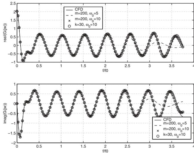
FIG. 4.11. Transfer function from incoming density perturbation to average throat Mach number for supersonic diffuser. Results from CFD model ( $n = 11,730$ ) are compared to 200th-order FMR models with  $\omega_0 = 5, 10$ . The  $\omega_0 = 10$  model is further reduced to  $k = 30$  via balanced truncation.
