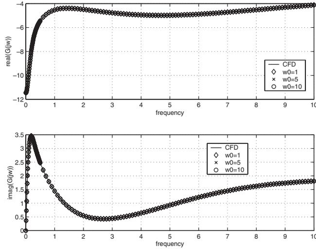
FIG. 4.1. Transfer function from plunging motion to lift force for subsonic airfoil. Results from CFD model ( $n = 13,928$ ) are compared to reduced-order models derived using 200 Fourier coefficients with  $\omega_0 = 1, 5, 10$ .
