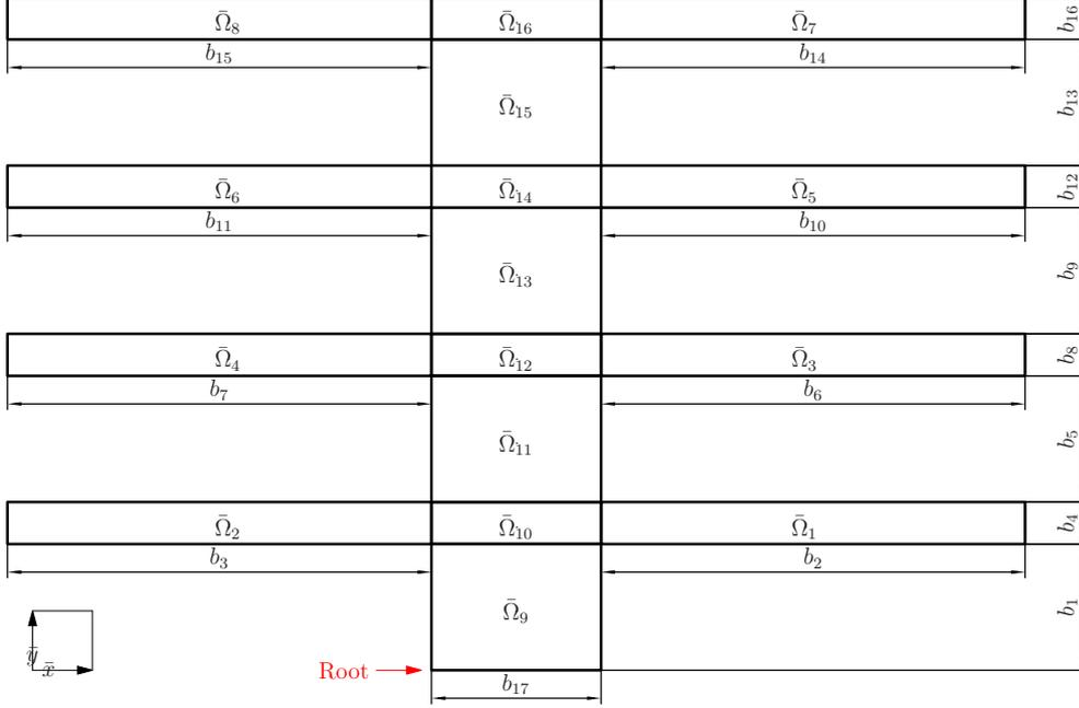
FIG. 5.1. The thermal fin geometry and subdomain definitions.
