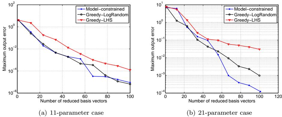
FIG. 5.5. *Model-constrained adaptive sampling approach versus greedy sampling approaches (Greedy-LogRandom: greedy sampling with logarithmic random trial parameter set; Greedy-LHS: greedy sampling with LHS trial parameter set) over 100 greedy cycles. A trial set with  $10^4$  parameter points is used in the greedy sampling approaches.*
