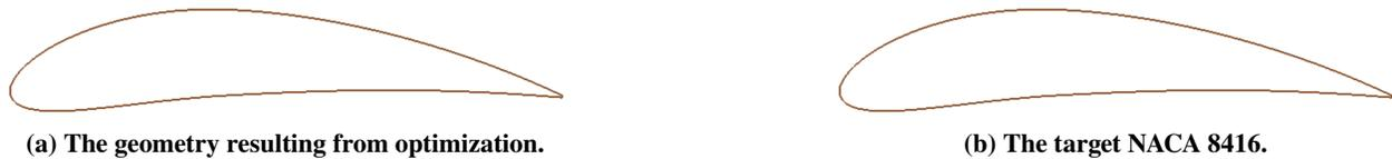
**Fig. 4** The resulting and target airfoils.
