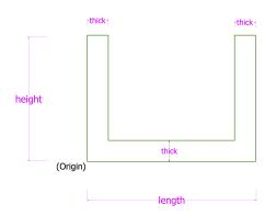
Measurements length = 4.00 height = 3.00 thick = 0.5
