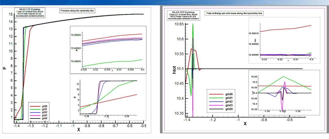
Pressure and total enthalpy along the symmetry line oscillation of total enthalpy of the order of 1 to 2 %
