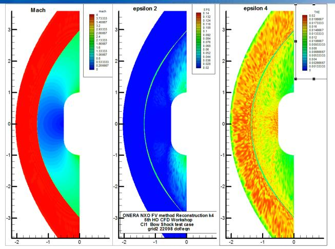
Iso\_Mach and coefficients of artificial dissipation ; discontinuity sensor based on variation of pressure across the stencil
