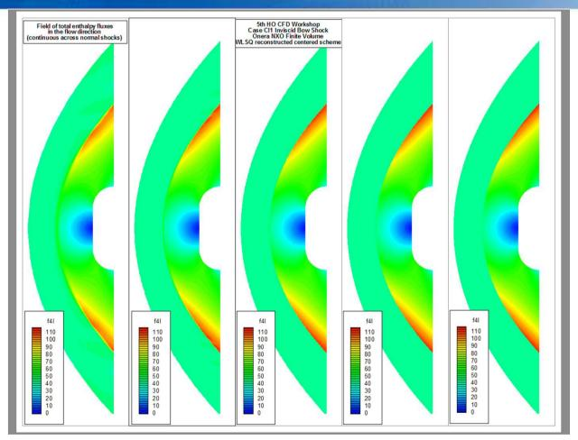
Field of fluxes in the flow direction for the energy equation (quantity interpolated at HO in the stencils across the normal shock
