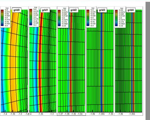
Shock location with respect to the grid refinement Field of total enthalpy
