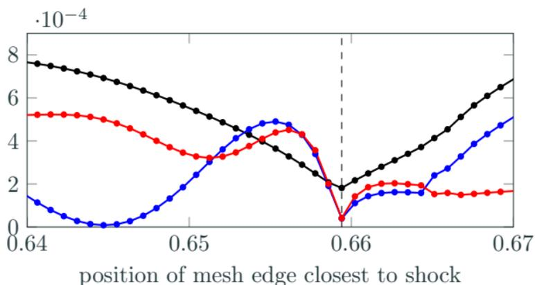
Objective function as an element edge is smoothly swept across shock location for:  $f_{shk}(\mathbf{u}, \mathbf{x})$  (—●—), residual-based objective (—●—), and Rankine-Hugniot-based objective (—●—).
