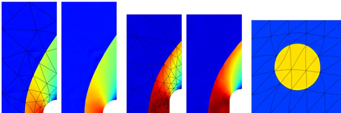
Mach 2 flow around cylinder (*left*), Mach 4 flow around blunt body (*middle*), and  $L^2$  projection of discontinuous function (*right*).
