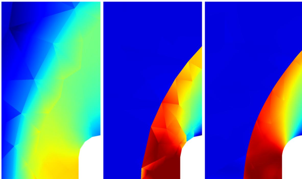
The solution of the CI1 bow shock problem. *Left*: Solution on non-aligned mesh with 102 linear elements and added viscosity (initial guess for shock tracking method). *Middle/right*: solution using shock tracking framework corresponding to mesh with 102 linear (*middle*) and quadratic (*right*) elements.
