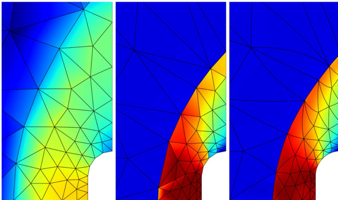
The solution of the CII bow shock problem. *Left*: Solution on non-aligned mesh with 102 linear elements and added viscosity (initial guess for shock tracking method). *Middle/right*: solution using shock tracking framework corresponding to mesh with 102 linear (*middle*) and quadratic (*right*) elements.
