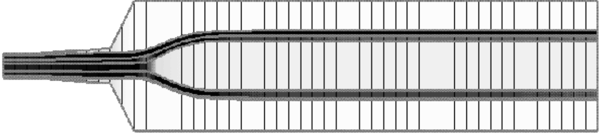
Figure 4-2: Flow Plot: Mach Number
