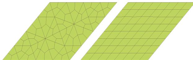
**Fig. 19** A flat surface with a non orthogonal boundary structure before and after mesh smoothing. The final mesh is structured and has uniform sizing but its internal angles are not in a  $90^\circ$  configuration.
