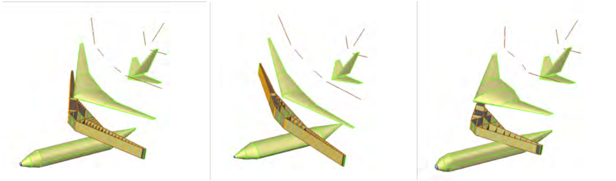
Fig. 1 Parametric variations of conceptual components embodied in a transport design model (components are separated for clarity, but are coincident in the actual model). Control surfaces are represented by their hinge lines, shown above the wing. Note that components vary consistently with respect to shared design parameters, which may include topological structure changes ( e.g. , number of ribs).
