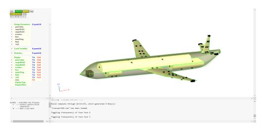
Fig. 14 Wing, horizontal tail, and vertical tail added to the configuration.
