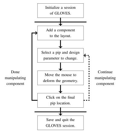
Fig. 7 Workflow in GLOVES for adding and manipulating components.
