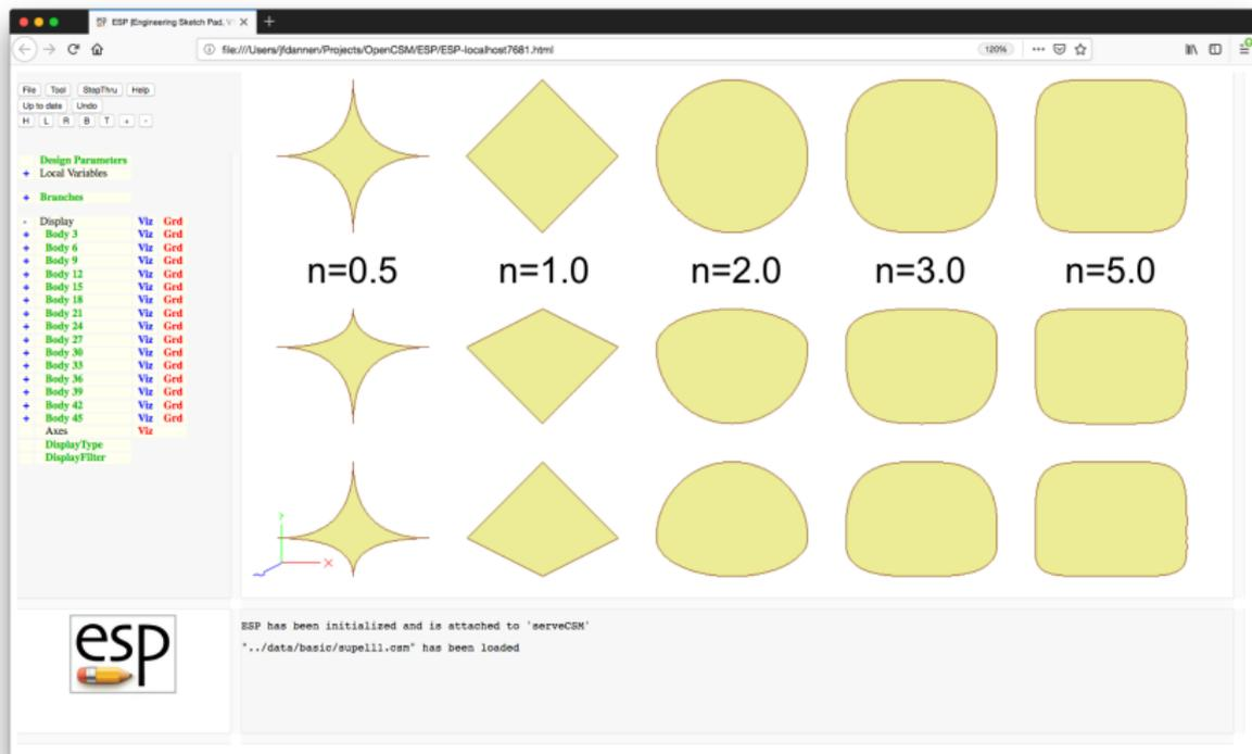
The screenshot shows the ESP (Engineering Sketch Pad) interface. The main workspace displays a 3x5 grid of super-ellipses, each labeled with a value of  $n$ :  $n=0.5$ ,  $n=1.0$ ,  $n=2.0$ ,  $n=3.0$ , and  $n=5.0$ . The shapes transition from a four-pointed star ( $n=0.5$ ) to a diamond ( $n=1.0$ ), a circle ( $n=2.0$ ), and finally to a rounded square ( $n=5.0$ ). A small 3D coordinate system is visible in the bottom-left corner of the grid.
