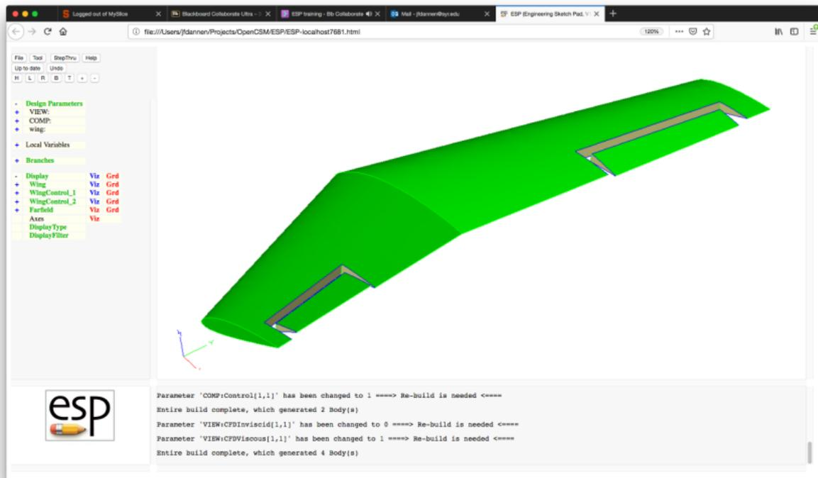
The screenshot shows the ESP (Engineering Sketch Pad) software interface. The main window displays a 3D model of a wing with two control surfaces. The wing is colored green, and the control surfaces are grey. The software interface includes a menu bar (File, Tools, Step Thru, Help), a toolbar, and a design tree on the left. The design tree shows the following structure:
