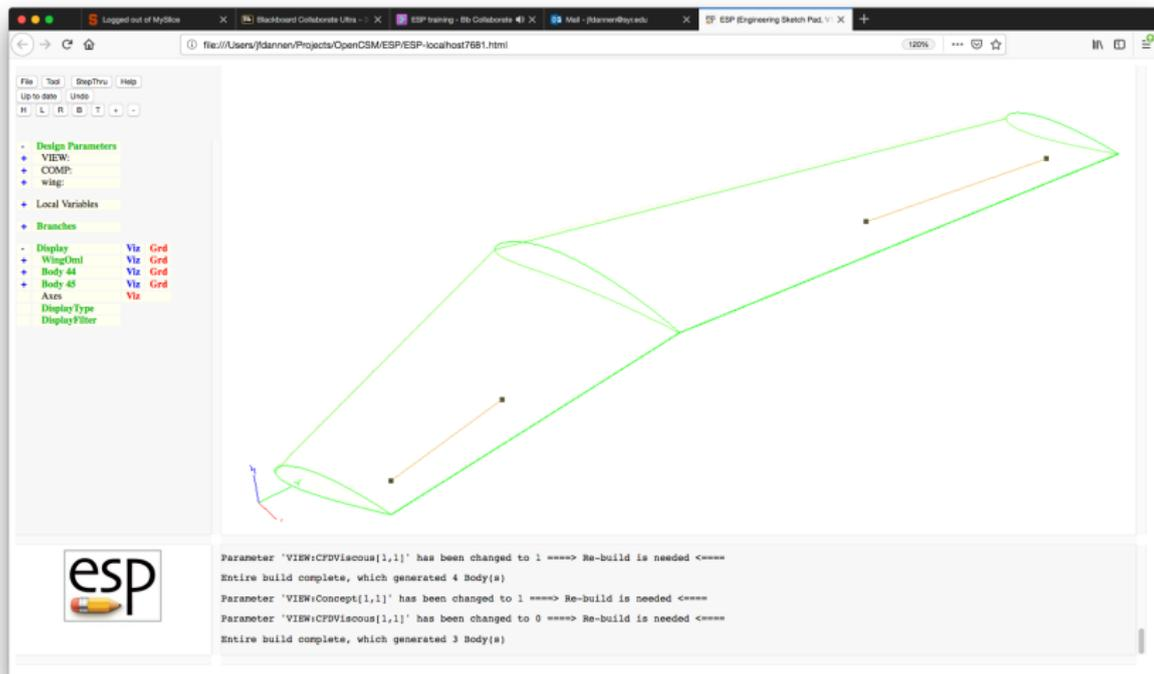
The screenshot displays the ESP Engineering Sketch Pad interface. The main workspace shows a 3D wireframe model of a wing with control surfaces, rendered in green. Two orange lines with black dots at their ends represent control surface actuators. A small 3D coordinate system is visible at the bottom left of the model.
